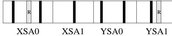
Figure 3: The composite signature of X bridged to Y with match restrictions (in black) and match requirements (labeled R)
